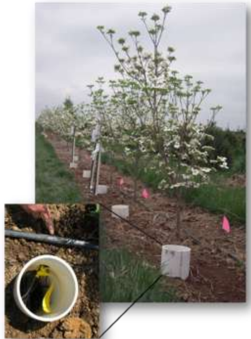
Figure 8. Decagon EM50R network on Cornus florida trees at Raemelton Farm. Insert shows sensors located in PVC tube in the root zone.
