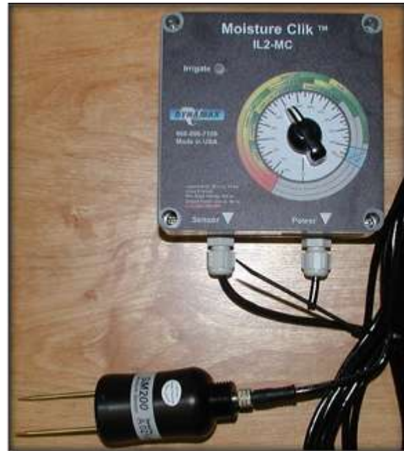
Figure 24. A MoistureClick irrigation controller
