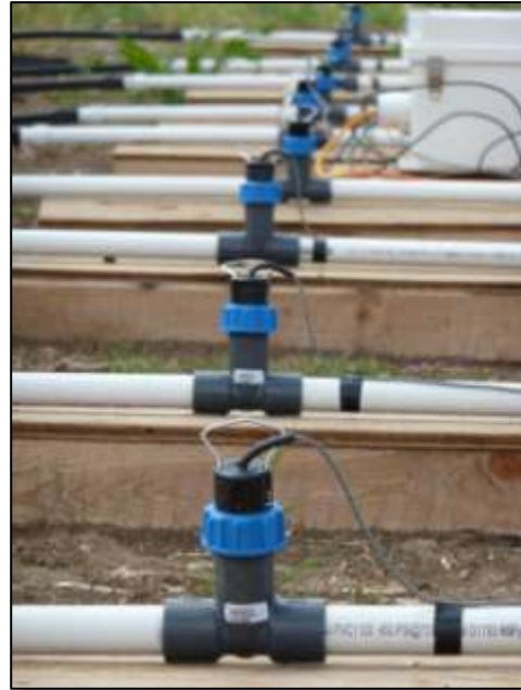
Figure 28 (A) Species specific solenoid irrigation control and (B) in-line species specific irrigation measurement.
