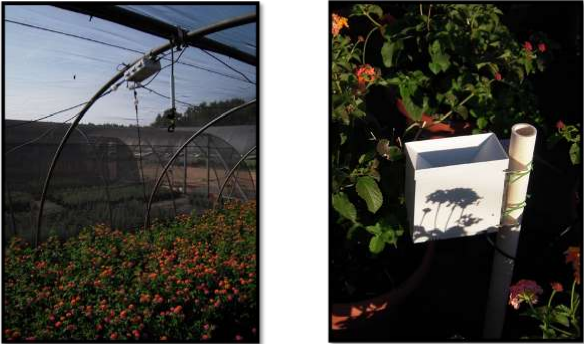
Figure 21. A Decagon EM50 datalogger is suspended above a lantana crop (left). Substrate moisture content in the crop is monitored using EC-5 sensors, while irrigation is monitored using a rain gauge (left) at Evergreen Nursery.
