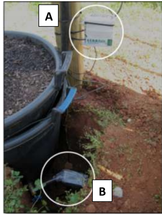
Figure 15. Installation of ECRN-50 rain gauges to measure (A) applied irrigation volume and (B) leachate volumes from the 30-gallon container.
