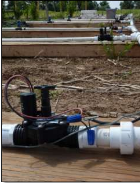
Figure 28 (A) Species specific solenoid irrigation control and (B) in-line species specific irrigation measurement.
