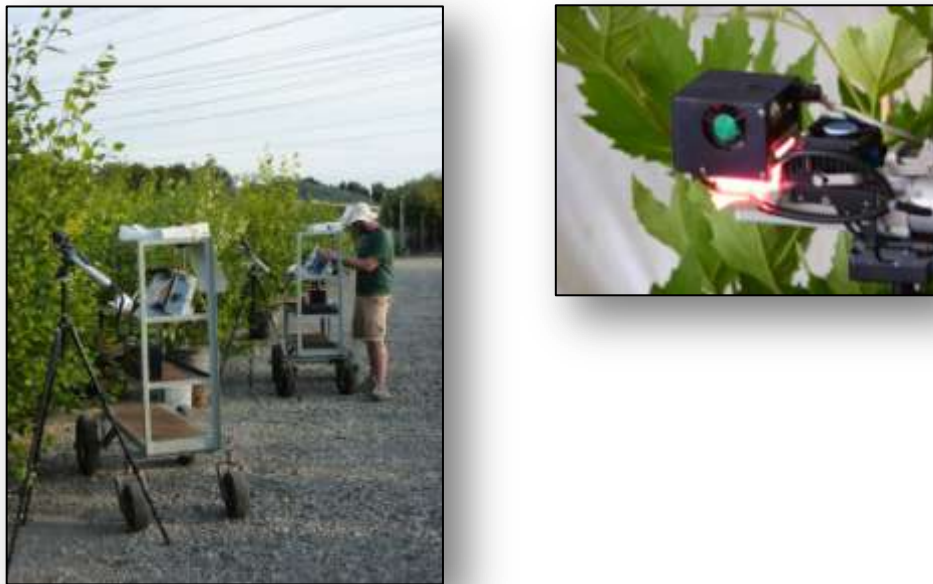
Figure 30. Dual gas exchange systems were used to collect the seasonal change in physiological parameters (model input) for ten species. Cuvette close up at right illustrates environmental control (e.g. light) for the characterization of species responses across variable environmental conditions.
