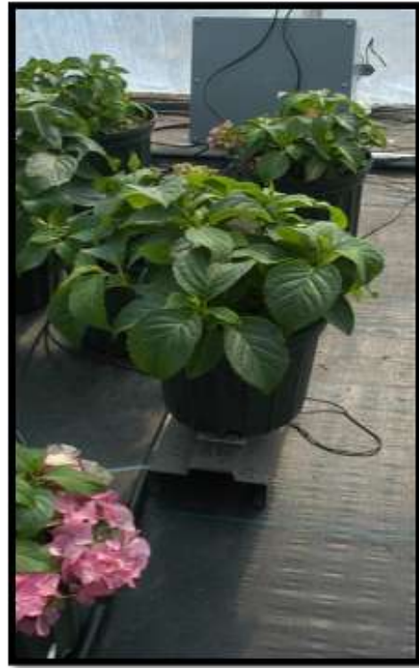
Figure 27. A hydrangea plant on a load cell to determine its daily water use.
