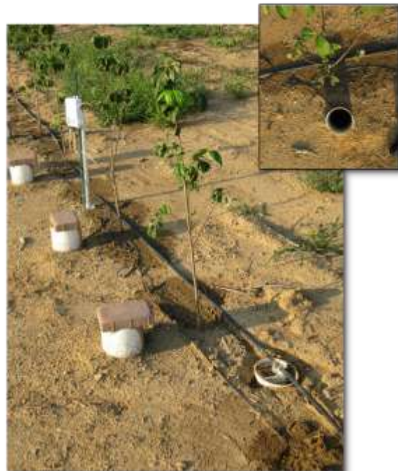
Figure 10. One-node network on four Cornus florida transplants; note the surface drip irrigation pattern from two emitters (top inset).
